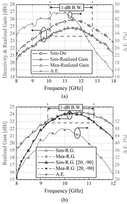
Fig. 5 Gain responses of (a) transmitarray functionality; (b) reflectarray functionality.
