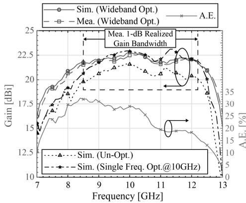
Fig. 8 Gain and aperture efficiency responses.
