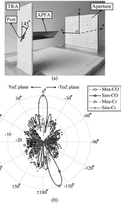
Fig. 6 (a) Photograph of AUT for bidirectional verification; (b) Normalized radiation pattern in YoZ plane at 10 GHz.
