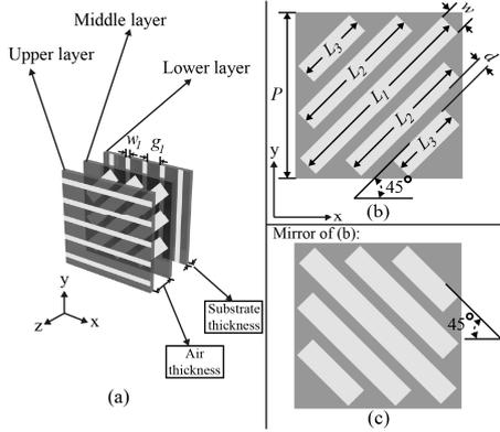
Fig. 7 Unit cell view (a) 3D view; (b) Middle layer of 0-bit element; (c) Middle layer of 1-bit element.  $L_1 = 18$ ,  $L_2 = 12.5$ ,  $L_3 = 6.5$ ,  $w = 2$ ,  $d = 1$ ,  $w_1 = 0.8$ ,  $g_1 = 2.2$ ,  $air\_thickness = 4$ ,  $substrate\_thickness = 0.8$  in mm.
