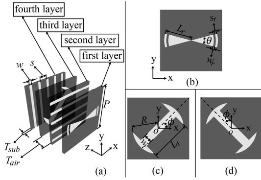
Fig. 4 Unit cell view (a) 3D view; (b) Top view of the first layer; (c) Top view of the third layer; (d) Mirrored structure of the third layer.  $s = 2.2$ ,  $w = 0.8$ ,  $T_{air} = 4$ ,  $T_{sub} = 0.8$ ,  $w_t = 2$ ,  $R = 6.2$ ,  $L_t = 1 \sim 12.2$ ,  $\theta = 30^\circ$ ,  $s_r = 0.5$ ,  $w_r = 0.5$ ,  $L_r = 2 \sim 7.4$  in mm.
