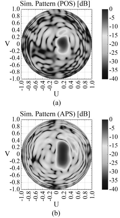
Fig. 3 Simulated Co-Pol radiation patterns ( $z > 0$ ) of (a) POS; (b) APS at 10 GHz.
