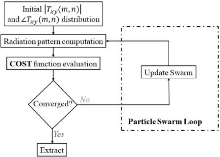
Fig. 2 Flowchart of the optimization loop.
