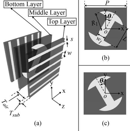
Fig. 1 Unit cell view (a) 3-D schematic; (b) Top view of the middle layer; (c) Mirrored structure of the middle layer.  $s = 0.8$ ,  $w = 2.2$ ,  $T_{air} = 4$ ,  $T_{sub} = 0.8$ ,  $w_1 = 3$ ,  $R_1 = 6.5, 6.8, 7.1$ ,  $\theta = 0^\circ \sim 45^\circ$ ,  $L = 1 \sim 12.8, 13.4, 14.0$  in mm.
