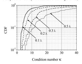
Fig. 6 CDF of condition number *K*-factor of the MSAA versus various array spacing in the Area 1.
