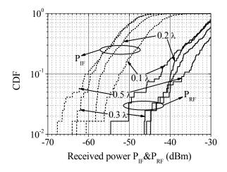
Fig. 3 CDF of simulated received power  $P_{RF}$  and  $P_{IF}$  of the MSAA versus various array spacing in the Area 1.
