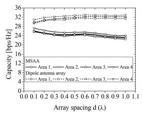
Fig. 9 Median MIMO channel capacity of the MSAA and the dipole array versus various array spacing in 4 different areas.
