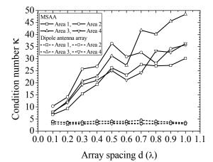
Fig. 7 Median condition number *K*-factor of the MSAA and the dipole antenna array versus various array spacing in 4 different areas.
