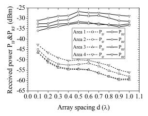
Fig. 4 Median results of simulated received power  $P_{RF}$  and  $P_{IF}$  of the MSAA versus various array spacing in 4 different areas.
