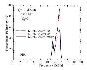
(a) Transmission efficiency versus Q when  $Q_n$  is 3
