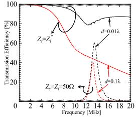
Fig.5 Transmission efficiency of two-dipole model
