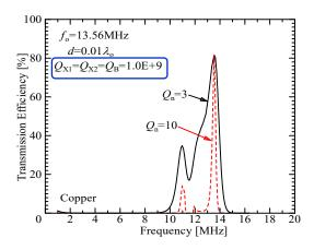
(b) Transmission efficiency versus  $Q_n$  when Q is 1.0E+9
