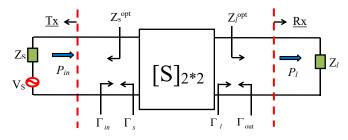
Fig.2 The equivalent circuit of two-port network
