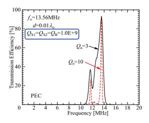
(b) Transmission efficiency versus  $Q_n$  when Q is 1.0E+9
