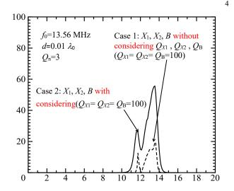
Fig.10 The transmission efficiency when with considering losses of matching circuit components and without the consideration.
