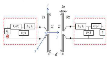
Fig.1 two-antenna WPT system with two-side lossy T-Section impedance matching circuits
