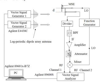
Figure 2: 2-channal MIMO measurement system
