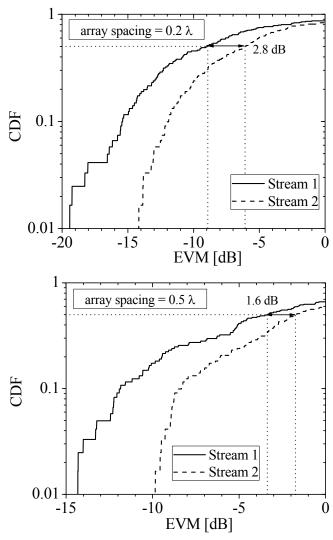
Figure 5: CDF of EVM of MSAA with the 0.2 and 0.5 wavelengths array spacing in the NLOS environment
