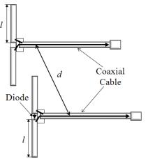
Figure 1: Geometry of modulated scattering dipole antenna array
