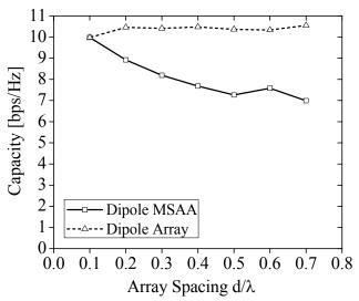
Figure 8: Median MIMO channel capacity of dipole MSAA and two dipoles antenna array versus various array spacing in the NLOS environment
