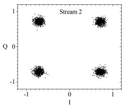
B) Constellation diagram of the stream 2 Figure 4: Constellation diagram of 2 streams demodulated from IEEE 802.11n signals received by MSAA
