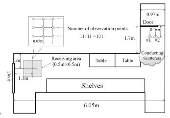
Figure 3: MIMO measurement environment
