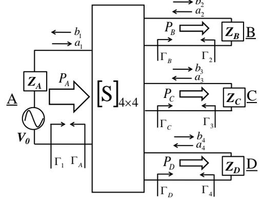
Fig. 1. 4-port network with 1 Tx port and 3 Rx ports.
