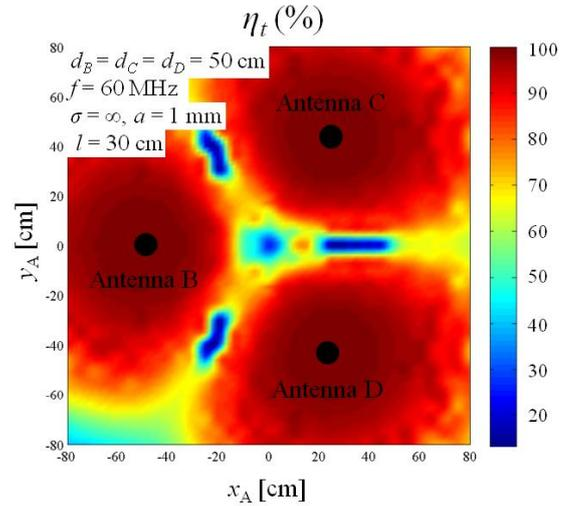
Fig. 7. The total PTE  $\eta_t$  when moving Tx antenna A
