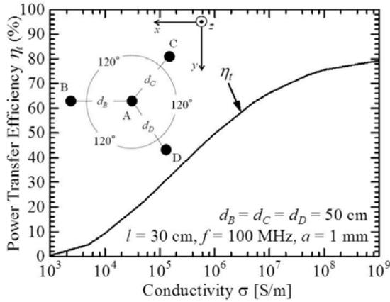
Fig. 4. PTE versus antenna conductivity.
