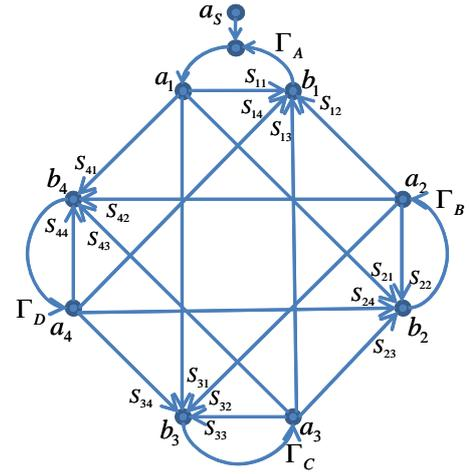
Fig. 2. Signal flow graph of 4-port network.
