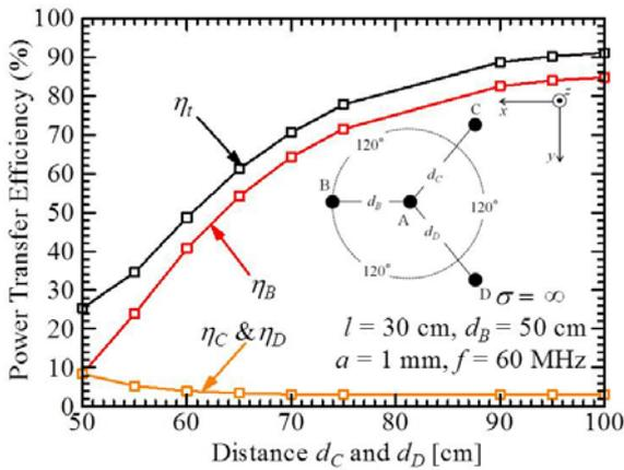
Fig. 5. PTE versus relative antenna positions in 60 MHz.
