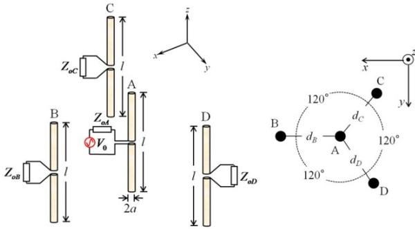
Fig. 3. Analysis model with 4 dipole antennas.
