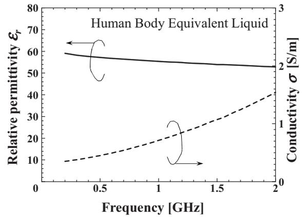
Fig. 2. Relative permittivity and conductivity of human body equivalent liquid.
