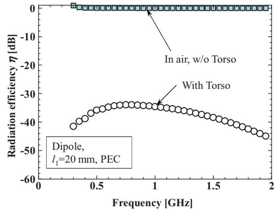
Fig. 3. Radiation efficiency of in-body antenna.
