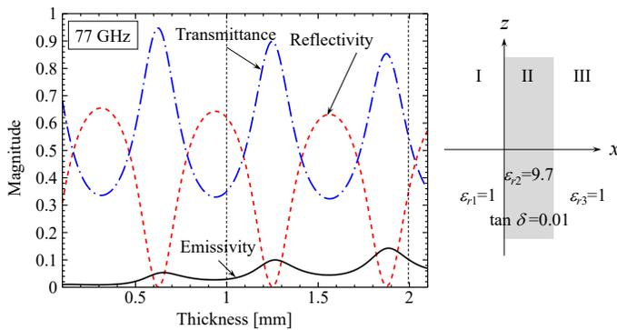
Fig. 5 Reflectivity, transmittance and emissivity as a function of the thickness of ceramic.
