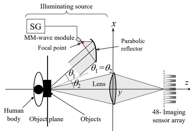
Fig. 1 Optical system of Sub-Active imaging.
