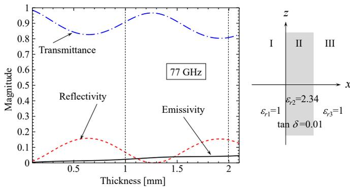
Fig. 4 Reflectivity, transmittance and emissivity as a function of the thickness of polyethylene.
