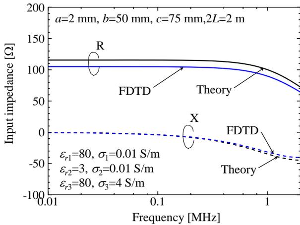
Fig. 3 Input impedance of full sheath dipole antenna with PVC-cover in seawater.
