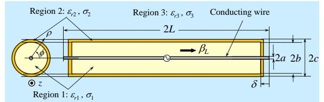
Fig. 1 Structure of sheathed dipole antenna with PVC-cover in seawater.
