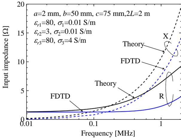
Fig. 2 Input impedance of half sheath dipole antenna with PVC-cover in seawater.
