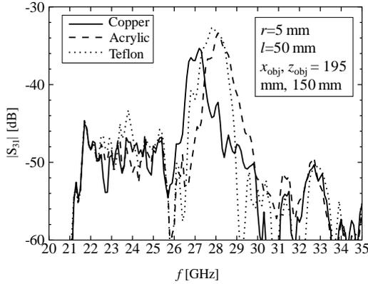
Fig. 3. One-dimensional detection of conducting and dielectric cylinders positioned in front of body phantom.
