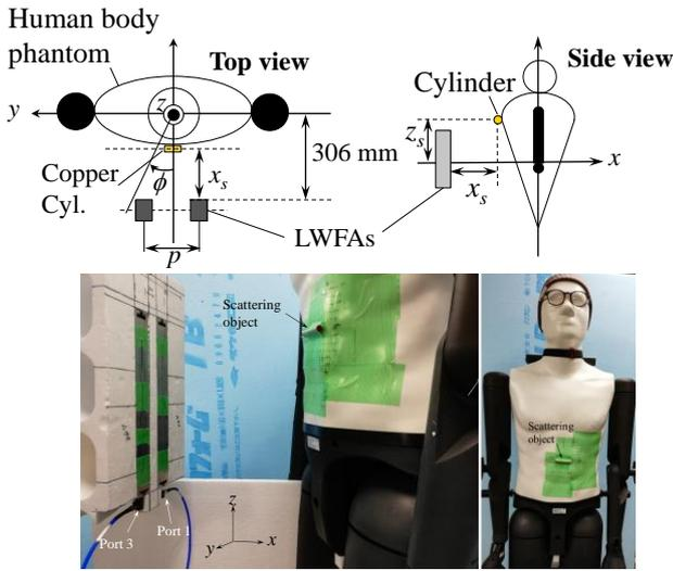
Fig. 2. Experiment setup with body phantom.
