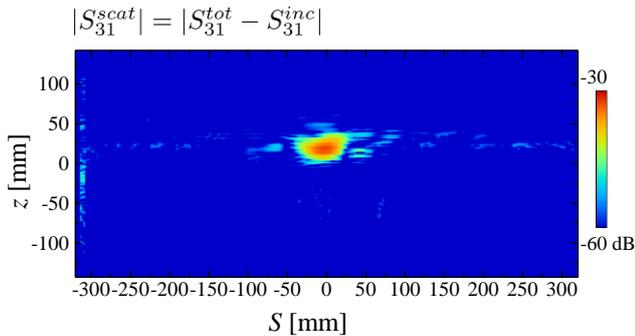
Fig. 4. Two-dimensional imaging of a copper cylinder positioned in front of body phantom before and after subtraction of incident field.
