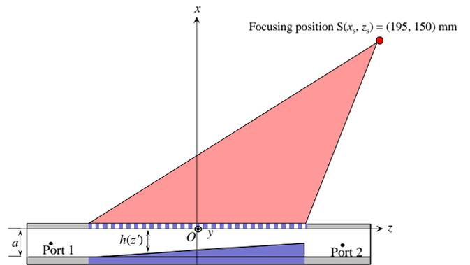
Fig. 1. Leaky-wave focusing antenna (LWFA) used in proposed system.
