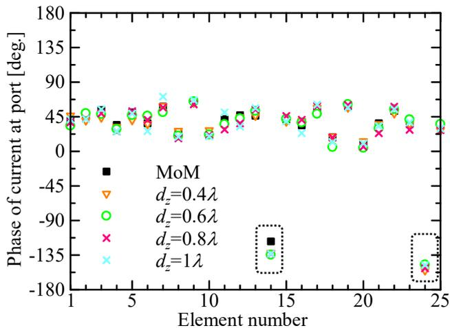
Fig. 2. Phase of current at port of loop array antennas (Dashed line indicates defective elements).
