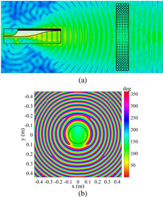
Fig. 4. (a). Simulated 2-D electric field distribution with APFA as source feed. (b). The aperture phase distribution at exit aperture plane. The black dot circle represents the actual physical aperture (0.189m diameter) of lens
