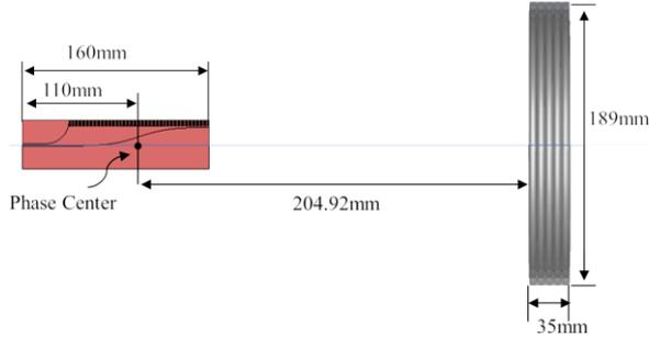
Fig. 3. The schematic of proposed H-S lens antenna at 10GHz composed of feeding source (APFA) and H-S lens. Fig. 4(a) illustrates the 2-D electric field distribution through the H-S lens. The aperture phase distribution at the exit aperture plane of the lens is given in Fig. 4(b). Obviously, proposed H-S lens can be a phase transformer to convert a spherical wave into a plane wave.
