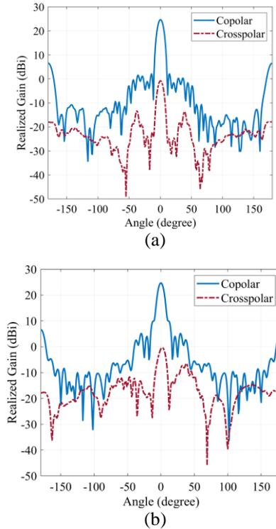
Fig. 5. Simulated co- and cross-polar radiation patterns in E-plane and H-plane respectively at 10GHz. (a) E-plane. (b) H-plane.
