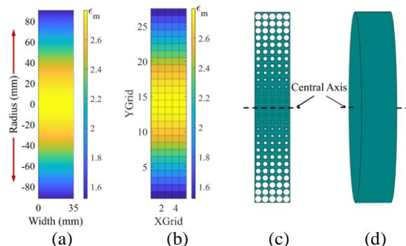
Fig. 2. The discretization of 2-D relative permittivity distribution of H-S lens. (a) Continuous distribution. (b) Discrete distribution. (c) Perforated dielectric structure. (d) Three-dimensional H-S lens
