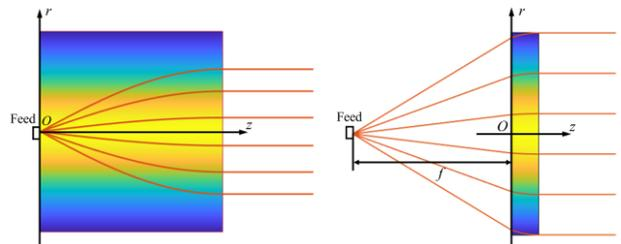
Fig. 1. The ray trajectory through the H-S lens. (a) Typical case of H-S lens. (b) Generalized H-S lens.
