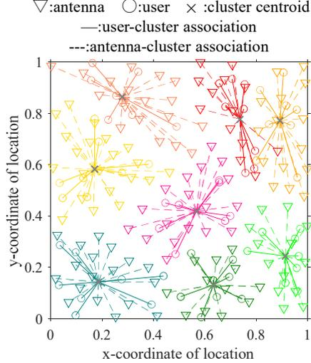
Fig. 1. An example of cluster structure after antenna assignment in a square-shaped single cell ( $U=64$ ,  $A=2 \times U$ ,  $AS=0.0625$ ,  $K=8$ ).
