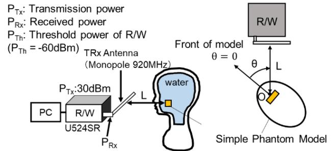
Fig.6 Measurement system of A (920MHz, in-body)
