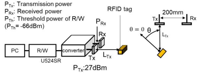
Fig.8 Measurement system of B (5.02GHz, out-body)
