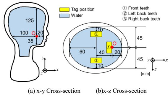
Fig.5 Cross sectional view of simple phantom model
