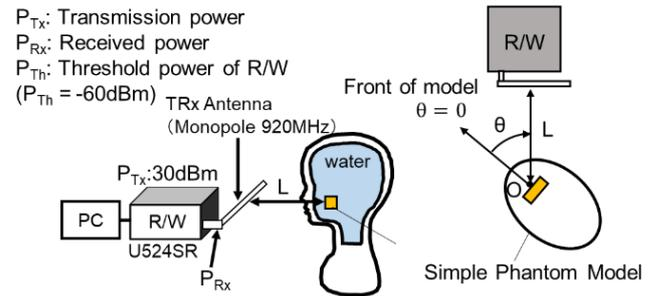
Fig.6 Measurement system of A (920MHz, in-body)
