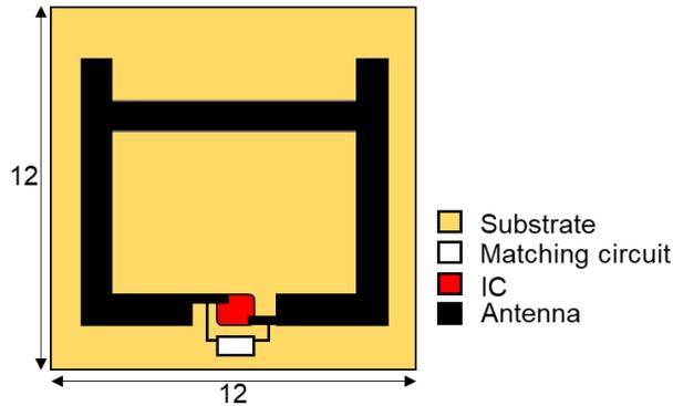
Fig.3 Structure of tag antenna. (Unit of length: mm)
