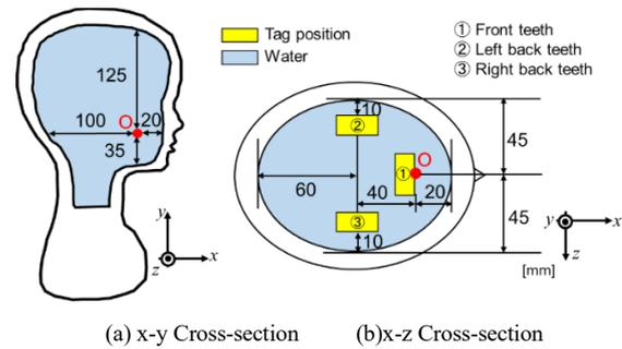
Fig.5 Cross sectional view of simple phantom model
