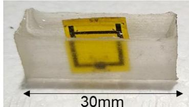
Fig.2 Photo of dual-use RFID tag embedded in resin block
