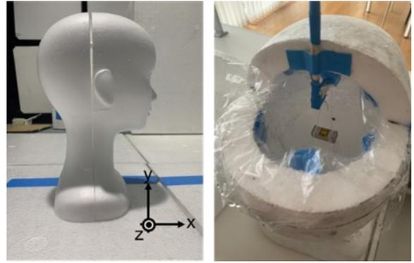
Fig.4 Photo of simple phantom model
