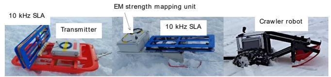
Fig. 14. The crawler robot towed the mapping unit (center) and the transmitter.
