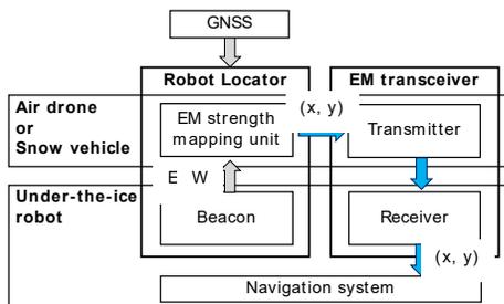
Fig. 1. System configuration of the UEML system.
