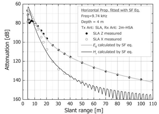
Fig. 8. Low frequency attenuation measured between air, sea-ice, and seawater in Saroma lake at 10 kHz.
