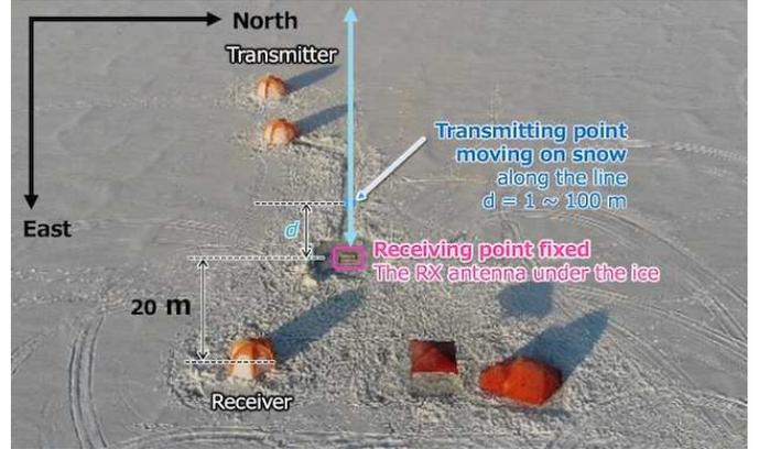
Fig. 4. Experimental configuration for horizontal propagation measurements in Saroma lake. Upper: cross-section view and lower: a snap shot of the test site in 2020.
