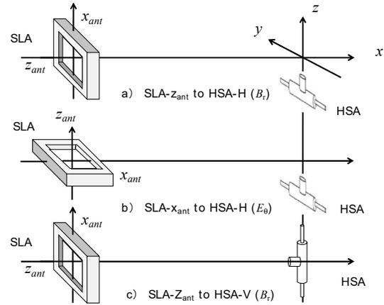
Fig. 5. Antenna polarization.
