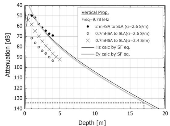
Fig. 9. An air-ice-sea boundary propagation in vertical at 10 kHz.
