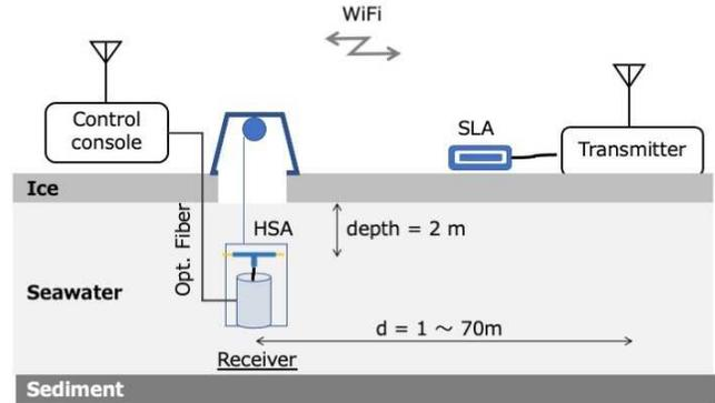
Fig. 12. Field set up of communication tests.
