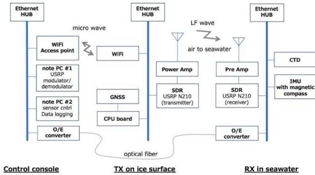
Fig. 10. Function blockdiagram of the function model for communication test
