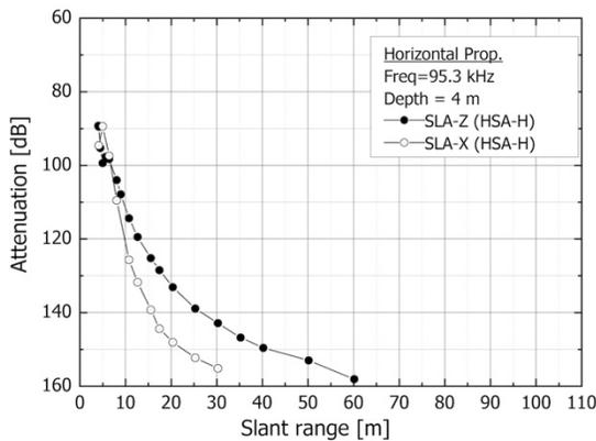
Fig. 7. Attenuation measured between air, sea-ice, and seawater in Saroma lake at frequency of 100 kHz.
