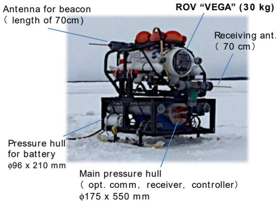
Fig. 13. The ROV equipped with the beacon, the antennas, and the pressure hulls.
