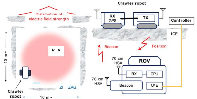
Fig. 15. An idea how to make a field strength map by the crawler robot and how to find a position of the underwater robot.
