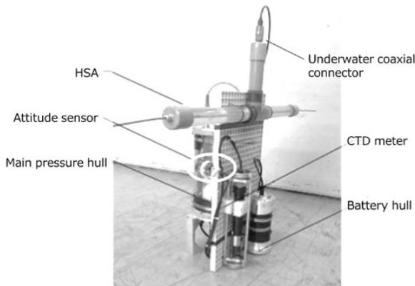
Fig. 11. An exterior view of the underwater receiver unit (RX). The 2 m-HSA is mounted on the top side of the frame. Its height is about 0.7 m and weight is about 20 kgs.
