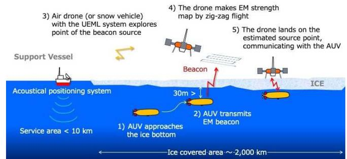
Fig. 2. An operation example of the localization with the proposed method.
