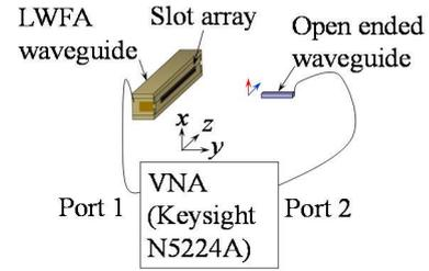
Fig. 2. Experiment setup to measure radiated component of electric field.
