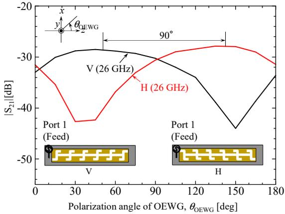
Fig. 4. Measured transmission coefficient between OEWG and LWFA for different polarization angles of OEWG  $\theta_{\text{OEWG}}$ .
