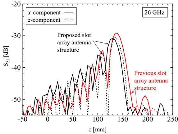
Fig. 3. Measured transmission coefficient between OEWG and LWFA with previous and proposed slot array antenna structure.
