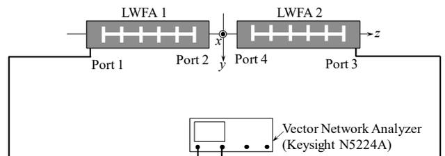
Fig. 2. Top view of experiment setup to measure the scattered and reflected field using leaky-wave focusing antennas (LWFAs).
