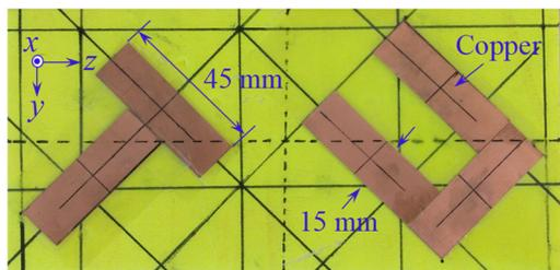
Fig. 3. Target object used in imaging experiment.
