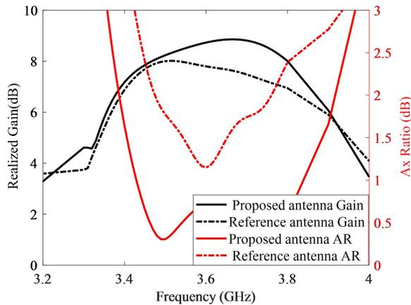
Figure 4 Simulated realized gain and axial ratio (AR) bandwidth ( $\phi=90^\circ$ ).
