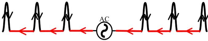
Figure 2. Current distributions of the proposed omnidirectional CP antenna.
