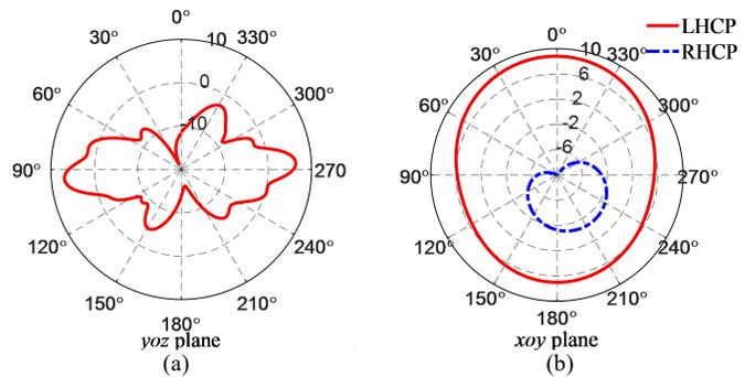
Figure 5. Radiation pattern of the proposed antenna at 3.7 GHz on (a)  $yoz$  plane; (b)  $xoy$  plane.
