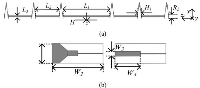
Figure 1. (a) Configuration of the proposed omnidirectional CP antenna; (b) Frontsize and backsize of balun.
