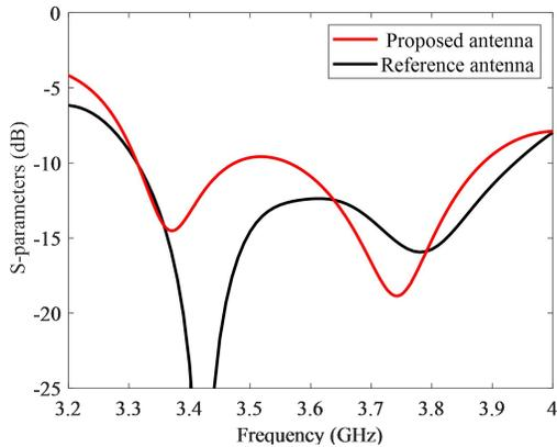
Figure 3. Simulated reflection coefficients of the proposed antenna and the reference antenna.
