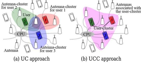
Fig. 1. CF-mMIMO system models using UC and UCC approaches for users 1, 2, and 3 of interest.
