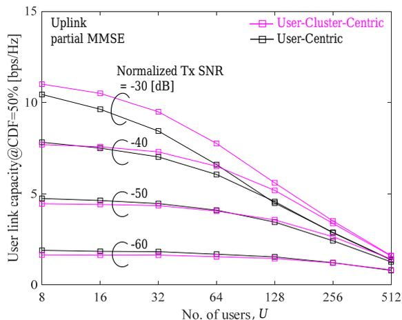
Fig. 5. User capacities achievable with the UC and UCC approaches.
