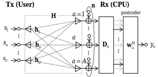
Fig. 2. Uplink transmission model assuming that user  $u$  belongs to user-cluster  $k$ .
