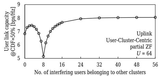
Fig. 4. Impact of the number of interfering users to be taken in the weight calculation of partial ZF.
