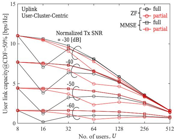
Fig. 3. User capacities achievable with ZF and MMSE postcoding.
