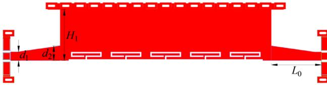
Fig. 6. Topology of the proposed BPF, where  $H_1 = 415 \mu\text{m}$ ,  $d_1 = 70 \mu\text{m}$ ,  $d_2 = 120 \mu\text{m}$ , and  $L_0 = 400 \mu\text{m}$ .
