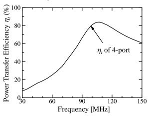
Fig.3 PTE frequency characteristics
